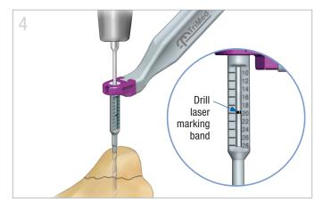
The following steps apply to the 2.3, 3.0, and 3.5mm screws. See Page 3 for technique on 1.7mm screws.
